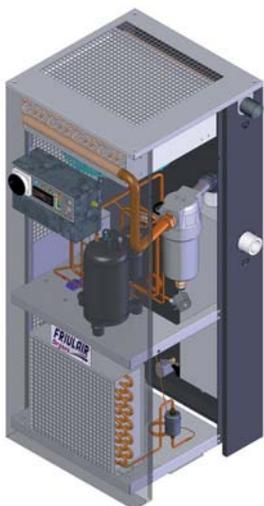
*AHT series includes an aftercooler, a pre-filter and a dryer in a single unit; and it is the modern evolution of a product already introduced in the market from Friulair, but update with latest technologies. This dryer combines a copper tube and aluminium fin air cooled aftercooler, a pre-filter with automatic drain and the established Alu-Dry Module Refrigerant Dryer, a completely aluminium heat exchanger built to a Friulair patented design. The product has numerous advantages:*
