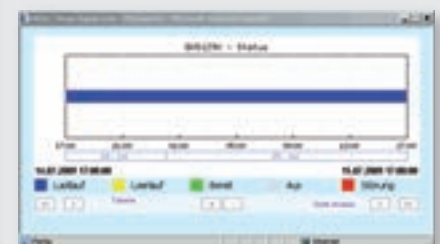
The status of each connected compressor can be visualised – additionally, the zoom-in and scrolling feature allows closer inspection and analysis of the acquired data.
