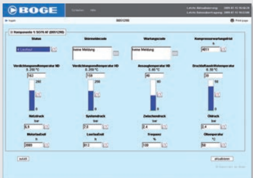
The web display shows all measured operating data at a glance, e.g. temperature, pressure, operating and idling hours as well as scheduled compressor maintenance intervals.
